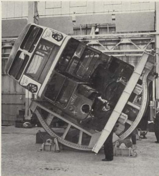
Fig. 2 Body underside being repaired on inverter
